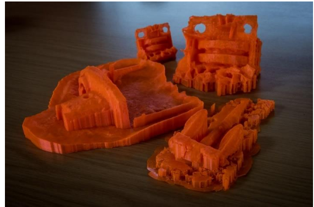
Examples of 3D printed shipwreck artefacts, achieved using underwater photogrammetry.
